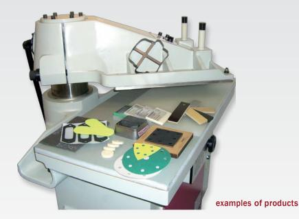
Depending on the requirements and intended application, swing arm cutting machines for manual insertion of material and tools are available in two basic designs. These machines are particularly suitable for small lot sizes or parts. All machine types listed are designed in a robust steel construction with a secure two-hand trip.
